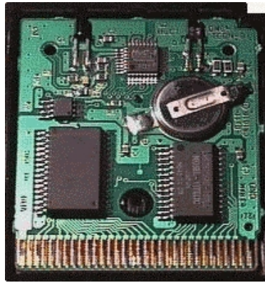
Figure 9: Game Boy Cartridge Circuit Board
