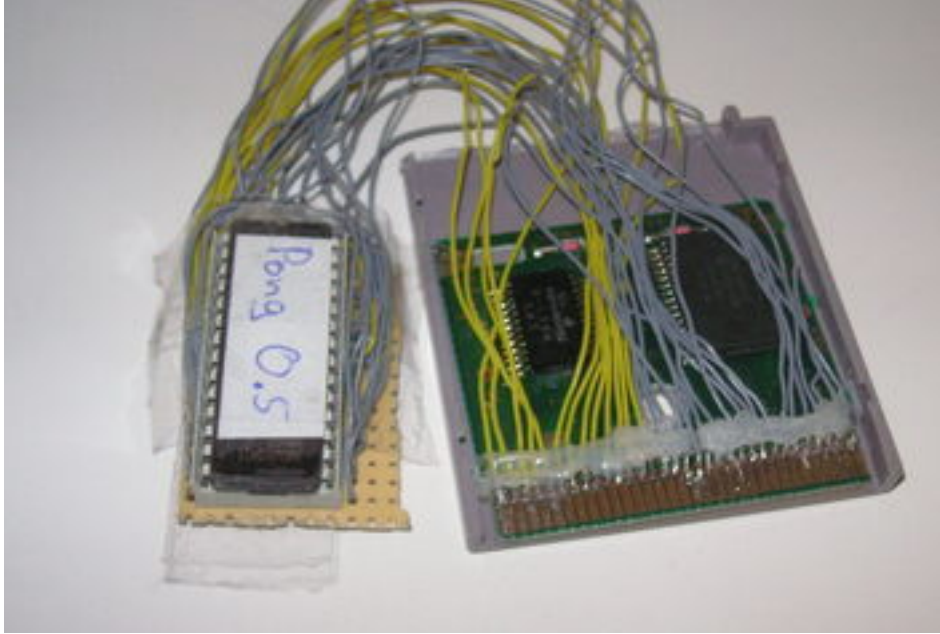
Figure 15: Modified custom Game Boy Cartridge connected to a 27C256
